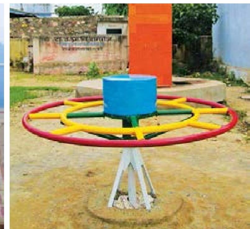
Merry go round pump: A technology that can ensure running water in schools
